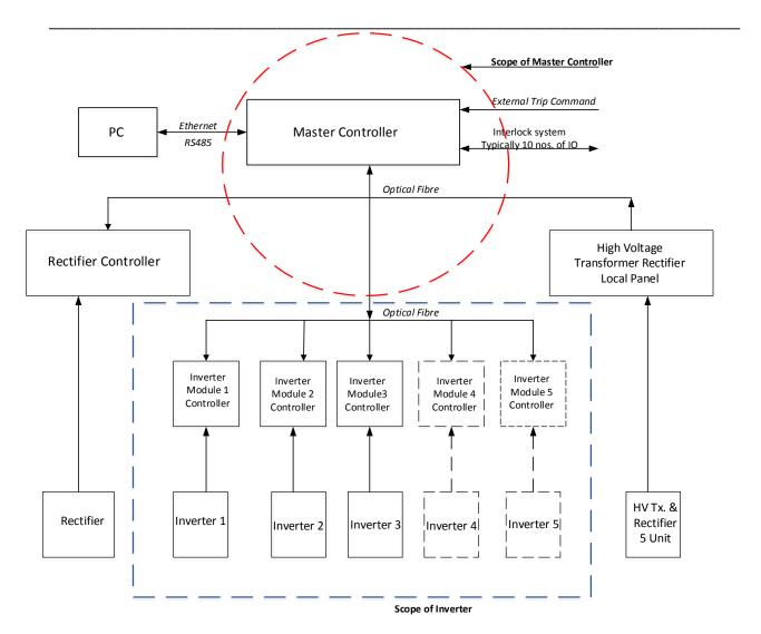
Figure-3: Block diagram of Control architecture of the 500kV UHVPS for reference only
