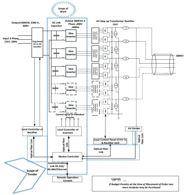
Remarks: All optical fiber link between local control panel to mater control panel including transmitter and receiver unit will be in the scope of Master Controller
